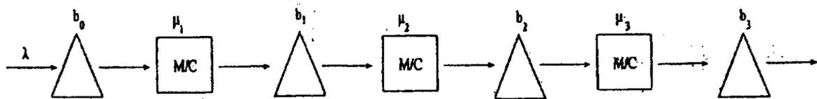
*Fig. Three machine-Two-buffer systems.*
